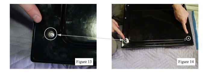
**Note: DO NOT** remove the four bottom hinge plate screws.
