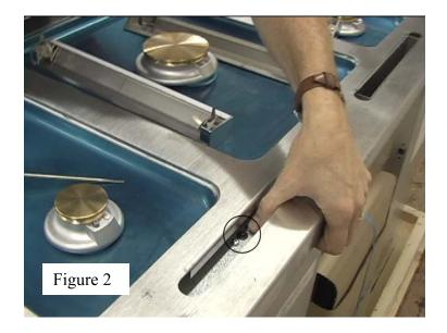
If your reset switch is not under the electric oven vent cover, you will need to lift the top of your range to access it.
