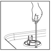
3 Two threaded spigots located under the air vent strip at either end hold the stainless steel table fixed to the control panel.
