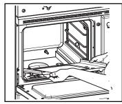
7 Using a 7 mm - 09/32" key, remove the screw that holds the burner.
