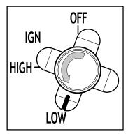
To turn off, turn the control knob clockwise to the OFF setting.
