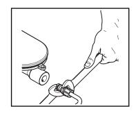
(10) Replace the seal and the injector.
