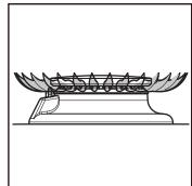
A reduced flowrate position (LOW) produces the preset minimum burner power (low flame).
