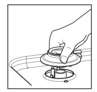
② Remove the fixing screws located under the burner bodies.
