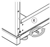
F Adjust the jacks using the 20 mm - 0<sup>25/32</sup>" spanner supplied.
