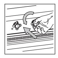
The low flame setting (LOW) delivers the pre-set minimum power from the burner.
