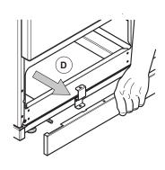
E Using the 7 mm - 09/32" in spanner supplied, turn the jacking screws. By doing this, the height of the appliance can be raised or lowered a few millimetres. The appliance can also be rested on the rollers, making it easier to move it to its final position.
