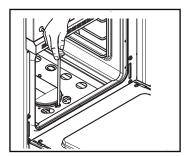
8 Remove the burner by pulling it towards the front and lifting its back.
