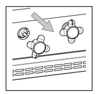
(3) Screw in or out the gas valve screw to adjust the delivery rate for the low flame. Screwing out increases the flame. Screwing in reduces the flame.
