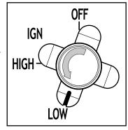
To turn off, turn the control knob clockwise to the OFF position.
